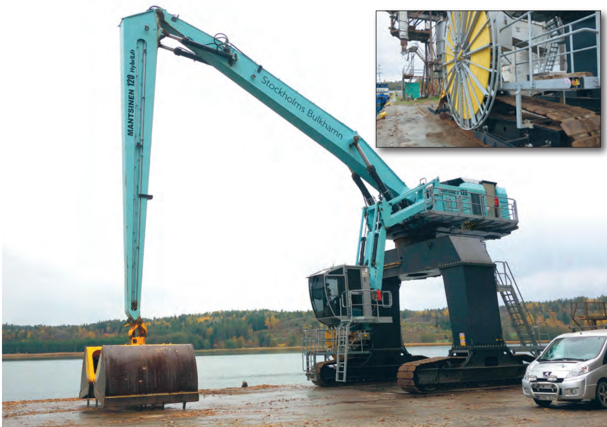
The port of Stora Vika has invested in an electrical harbour crane, and harbour manager Milan Tomich is very satisfied. "Because it's run on electricity, the crane is much quieter, which is important for us, as people living nearby have previously complained about noise. The cable can be a problem, but since we were able to specify the machine to 690 V (instead of the standard 450 V), the cable is relatively thin, which makes things easier."
