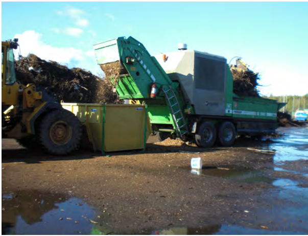
Willibald 5000 grinding logging residues.
