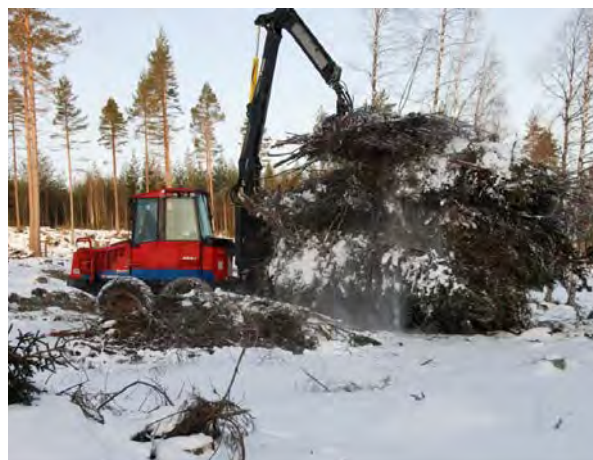
Forwarding of logging residues with conventional forwarder.
