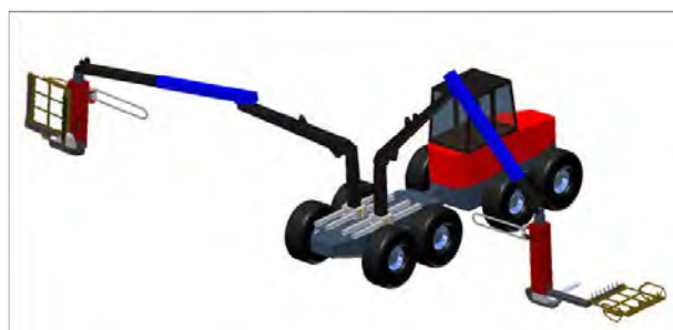
Concept sketch of a specialized boom corridor harvester that would enable profitable operation even in stands with mean diameters as low as approximately 6 cm dbh.
