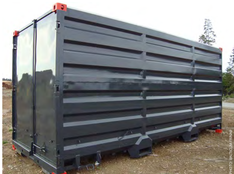
Conventional truck container where the tunnels for the forks can be seen under the container.
