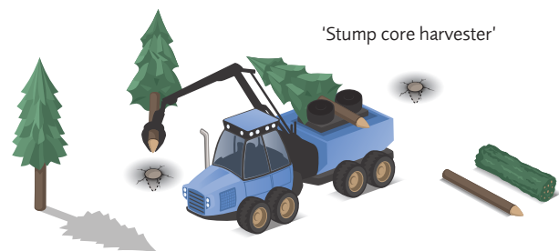
Design sketch of 'stump core harvester', which also produces logging residue bundles directly at the logging site. The stump unit cuts off the tree's lateral roots and then twists and lifts the tree up. On the ground behind the machine are a logging residue bundle and a butt log with associated stump core. Sketch based on a concept by Tomas Nordfjell.
