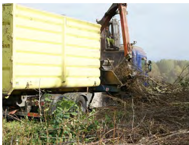
Chipper truck with Bruks's 805 chipper working with logging residues.
