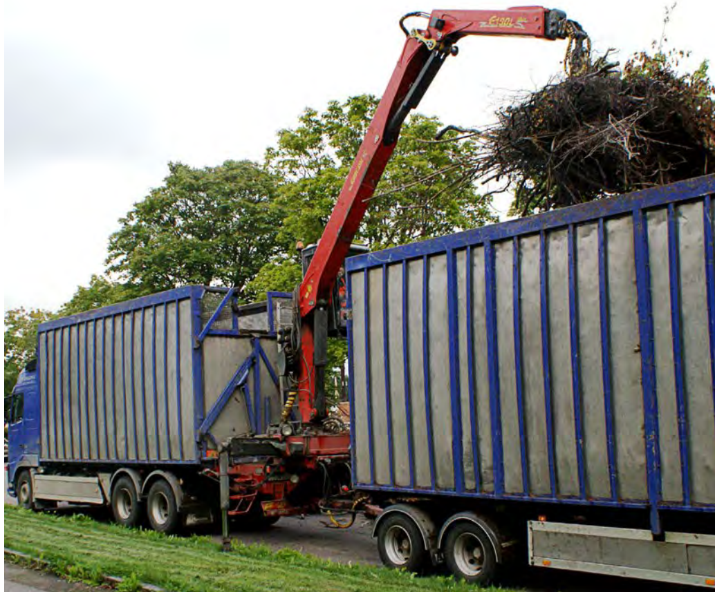
The loose logging residue system is competitive on short to medium-length distances. However, the relatively low payload is a weakness.
