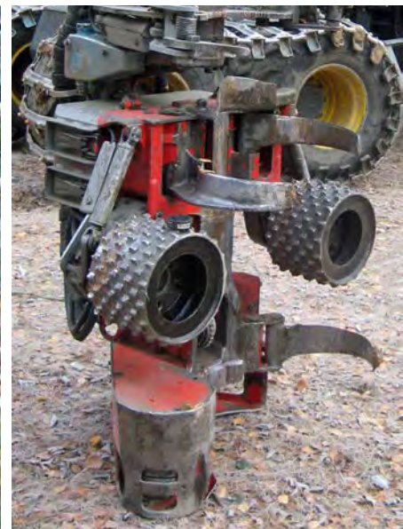
Log Max 4000. Harvester head with circular saw and feeder rollers. The accumulator function is reliable.
