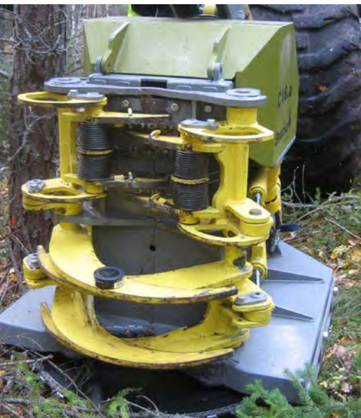
Bracke C16. Felling head with circular saw. The unit lacks feeder rollers. The accumulation function is relatively reliable.
