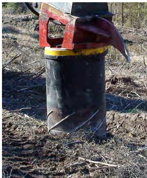
The rotary stump cutter loosens the stump by cutting off the lateral roots with the rotating drum.
