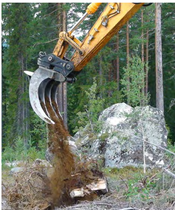
In terms of design, the Aalto fork is the simplest of the stump harvesters. It is mounted directly in the quick coupler attachment, and requires no extra hydraulics.
