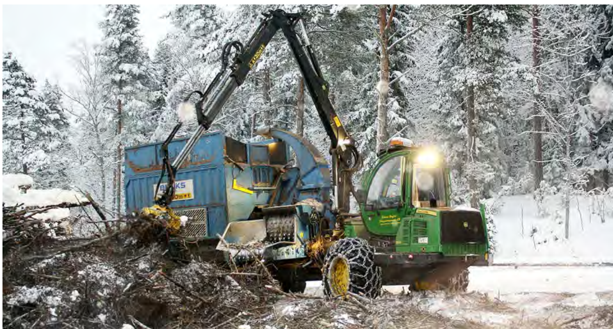
Chipping at the landing using forwarder-mounted chippers is common. A disadvantage of the system is the cost of moving the equipment between logging sites.
