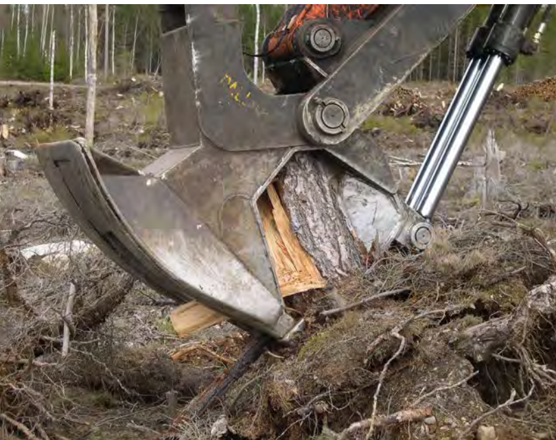
Pallari 140 is a shear-type unit. It is easily mounted in the excavator's bucket quick coupler attachment, and requires no special adaptations before mounting.
