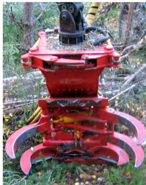
Naarva-Grip 1500-40E. Felling head with shears. The unit lacks feeder rollers. The accumulation function is reliable.
