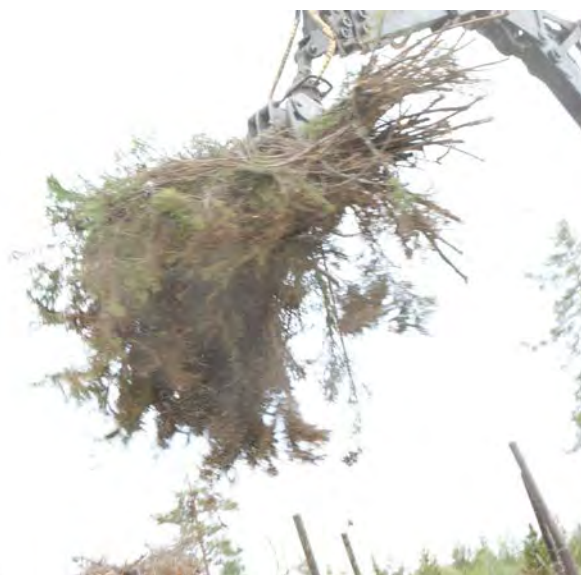
When loading logging residues the assymetric grapple forces the residues to form a sheaf-like, structured bundle.
