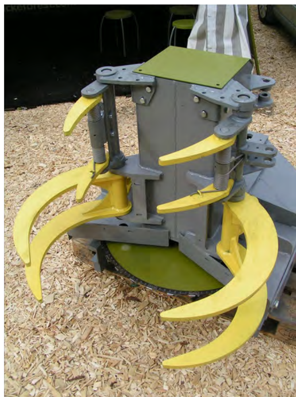
An early model of the Bracke C16a, the market's perhaps most advanced felling head for geometrical harvest in young, dense stands. Using this unit for felling and accumulation in stands with very thin trees, production can already reach approximately 4.5 tonnes DM/G 0 -hour (9 m 3 solid biomass/G 0 -hour and 500 trees/G 0 -hour). PHOTO: Tomas Nordfjell, SLU.
